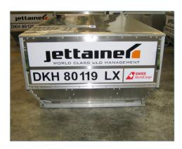
**DKH container** with steel doors used on narrow body aircraft A319/A320/A321. ULDs are secured with steel seals.
