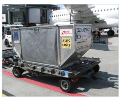
**DZH container** with steel doors used on narrow body aircraft A319 only. ULDs are secured with steel seals.
