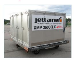
XMP/XKN container with steel doors used on wide body aircraft B77W/A330/ A340. ULDs are secured with steel seals.
