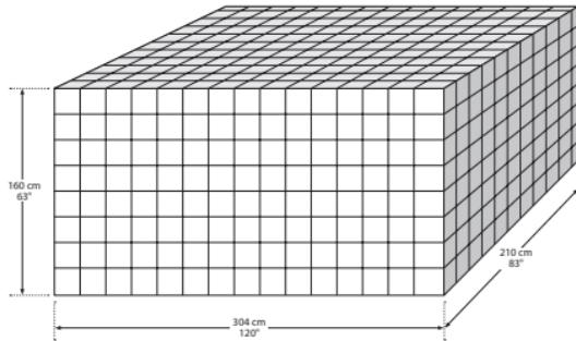
Weights depend on the structural weight limitations of the different pallet/container positions in the aircraft.
